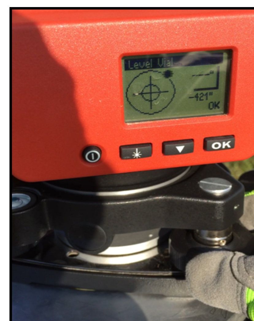
Figure 6. Total station accuracy must be adjusted for fractions of a millimeter
