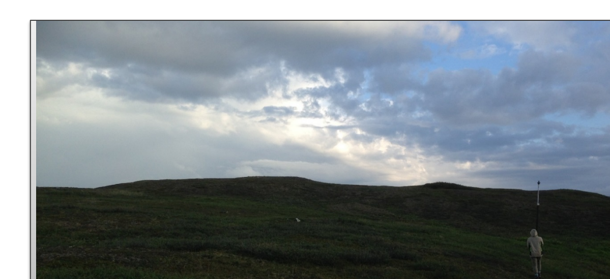
Figures 4 and 5. Prism rod is carried across lake and hills, while maintaining infrared signal from total station
